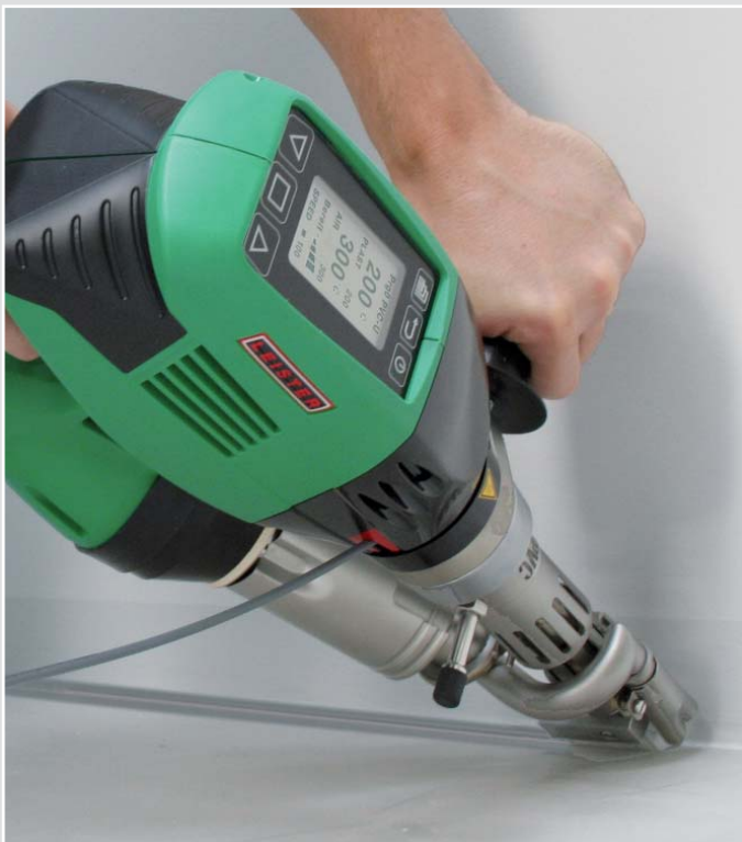
Despite its small size, the compact device produces up to 2.7kg of extrudate an hour.
